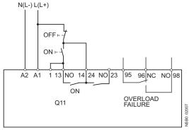
Control of a main contactor
