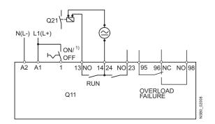
Connection example of 3RW40 2. ... 3RW40 4. for PTC sensors (thermistor motor protection) Thermoclick PTC type A
